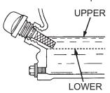
Figure 16. Engine Oil Dipstick (Oil Level)
